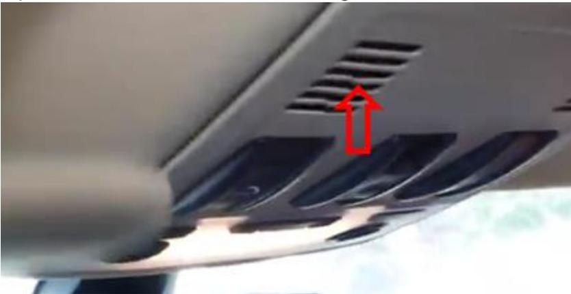
*Loosen the light unit by first unscrewing the clamps of both sun visors and pulling the cover down a bit. From the rear, push the light unit out of the rebate. You can now reach the microphone.
