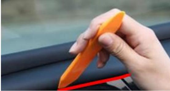
*Press the microphone cable under the cover strip with a spatula without damaging it or kinking it unnecessarily.*
